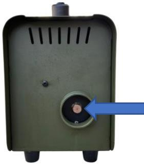
3. If the machine is still not running smoothly after nozzle cleaning, run a small amount of distilled water through the machine. Please make sure the water is completely out of the machine before performing your next treatment.
