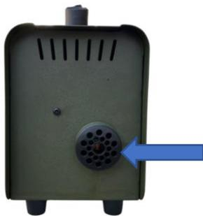
2. When the machine is cooled down, use an 11mm wrench or socket to remove the stainless-steel nozzle. Clean the nozzle with warm water to remove any debris blocking the pin hole in the center of the nozzle. Screw nozzle back onto the machine and reinstall the black plastic cover.
