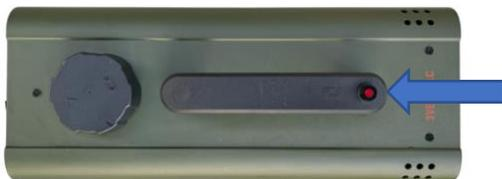
3. The machine is now ready to use. The machine has a built-in 30 second timer. When pressing the red button (On/Off Switch) on the handle once, the machine produces 30 seconds of treatment (1,000 sq ft), and then stops automatically at the end of 30 seconds. To stop the machine sooner, press the button on the handle, and the machine will stop. NEVER run the machine without solution in the tank.
